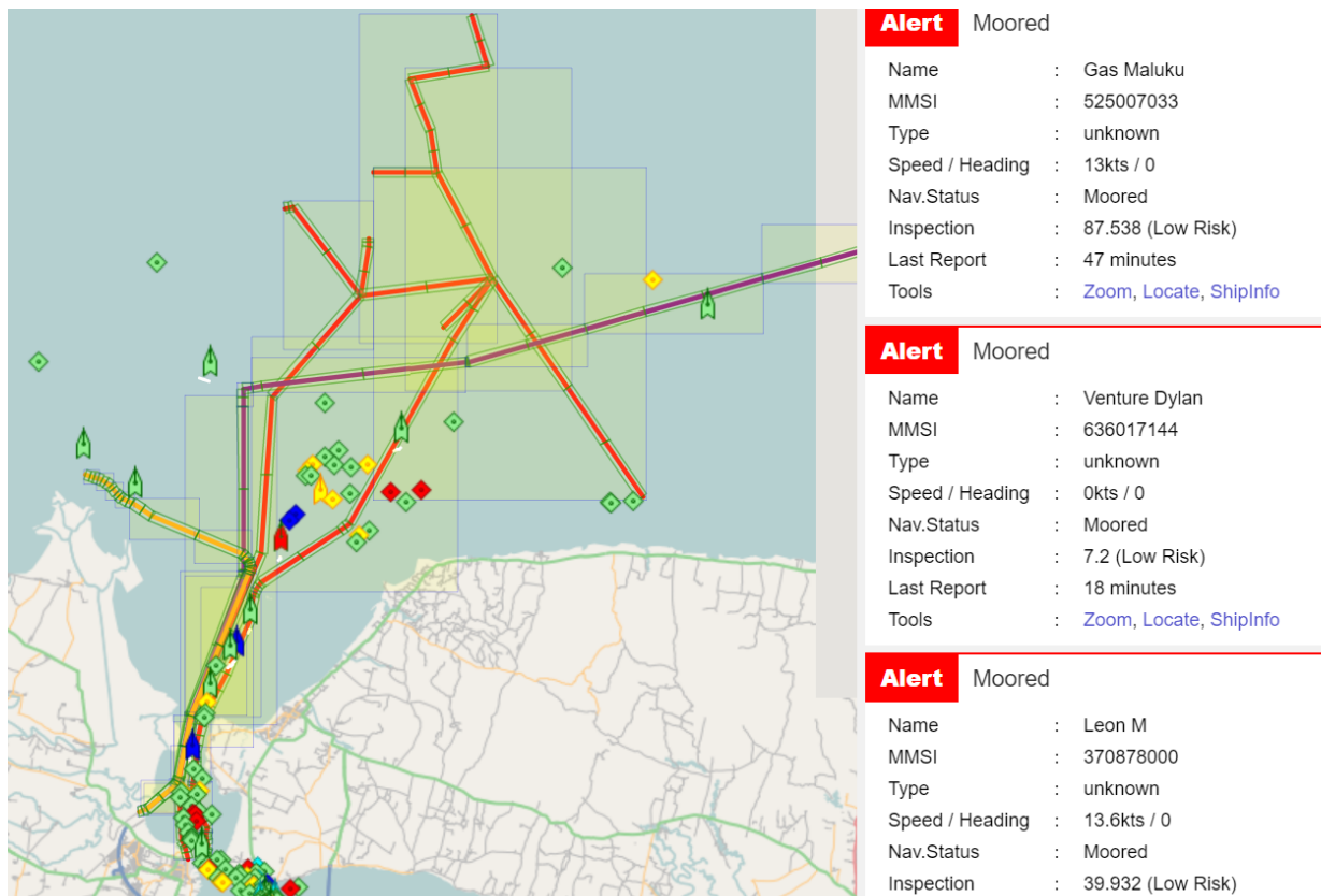
Figure 3: AISITS Pipeline Early Warning System (PEWS).
